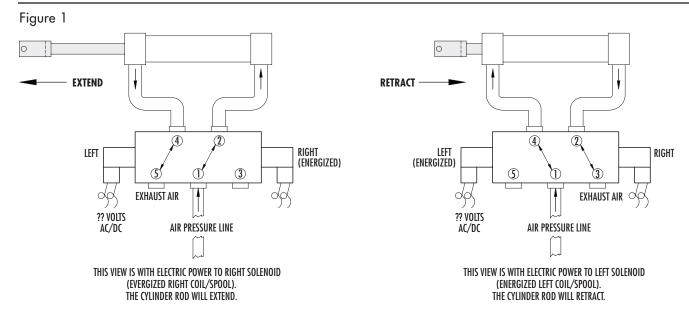
The double solenoid valve shown here is recommended for use on R&P Valves.
