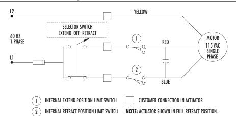
LIMIT SWITCHES ARE THE ONLY DEVICES PROVIDED. ANY STARTER, PUSH BUTTON CONTROL OR INDICATOR LIGHTS ARE TO BE SUPPLIED BY CUSTOMER.
